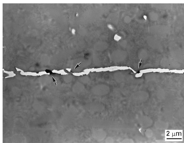
Figure 8 TEM micrograph taken at the DN-4PB damage behind the crack tip of LCE-2. When the main crack opens up, the matrix material between the segmented crack acts as a bridge (see arrows) to resist crack propagation.
